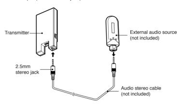
Figure 3: Use the DGL373 with alternative audio source
